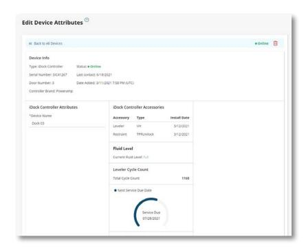
Check equipment serial numbers, installation dates, and leveler cycle counts online or on an iDock Controller.
