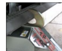
The TPR hook rotates up to engage the RIG and secure the trailer to the loading dock.
