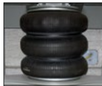
Steel-belted rubber bellows system uses compressed air to raise platform.
