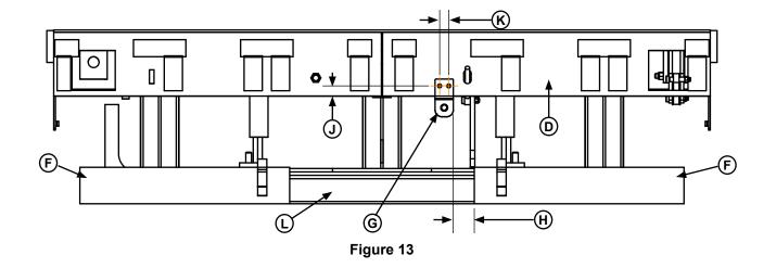
A— Tag Out Device D— Header G—Mounting Bracket K— Bracket Hole Spacing
