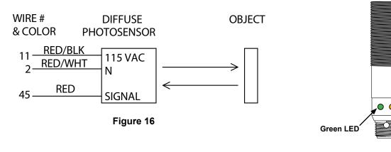
Green - Powered on Amber - Sensing target Flashing Amber - Partial Signal
