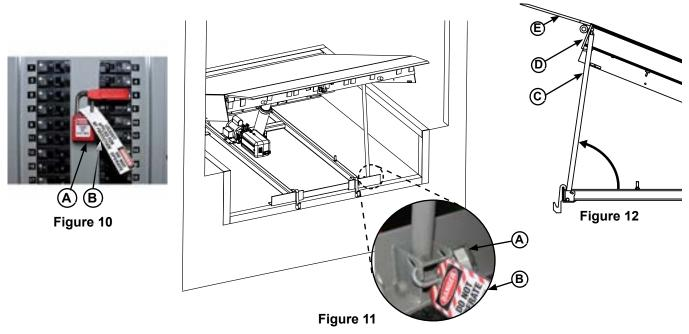
A — Lock Out Device C — Maintenance Prop E — Lip plate B — Tag Out D — Header plate
